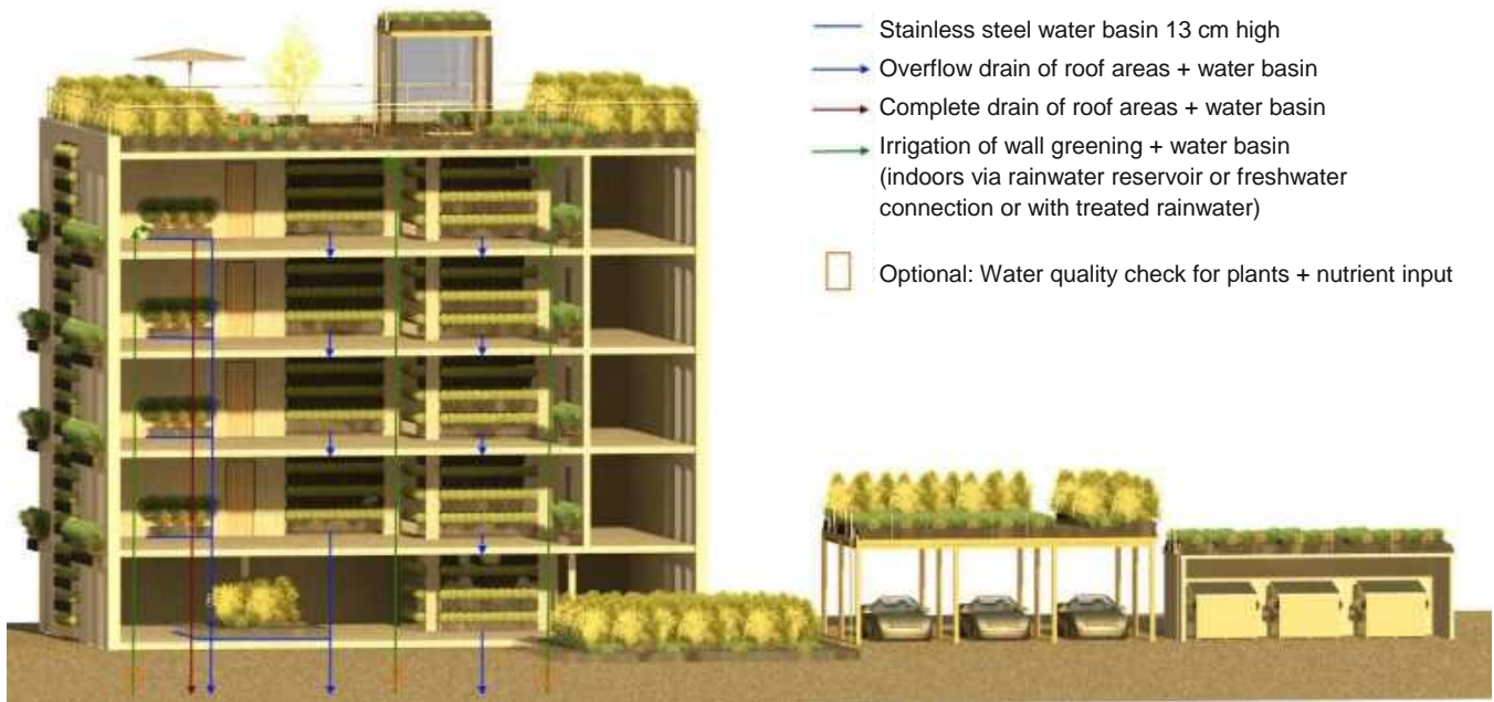
HPL® Systems for Building Greenery – water supply for indoor greening (for details see page 7)
