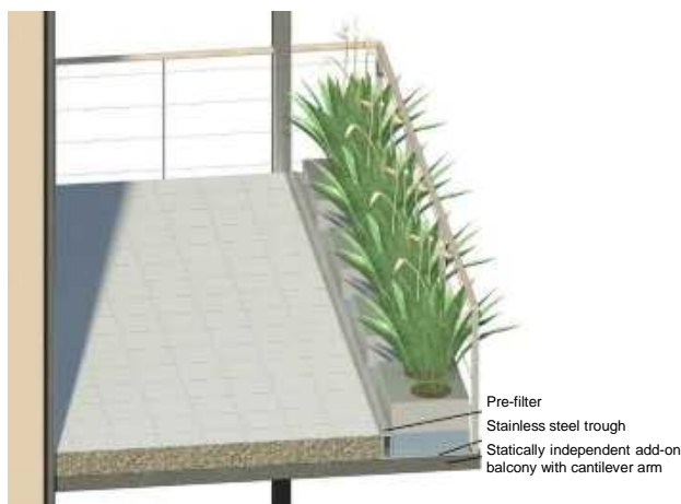
Fig. 3: Balcony new building / tiles on concrete – floor modules Installation of water basin
