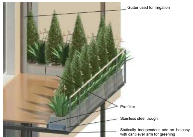
Fig. 4: Balcony new building / floorboards – floor modules Installation of water basin
